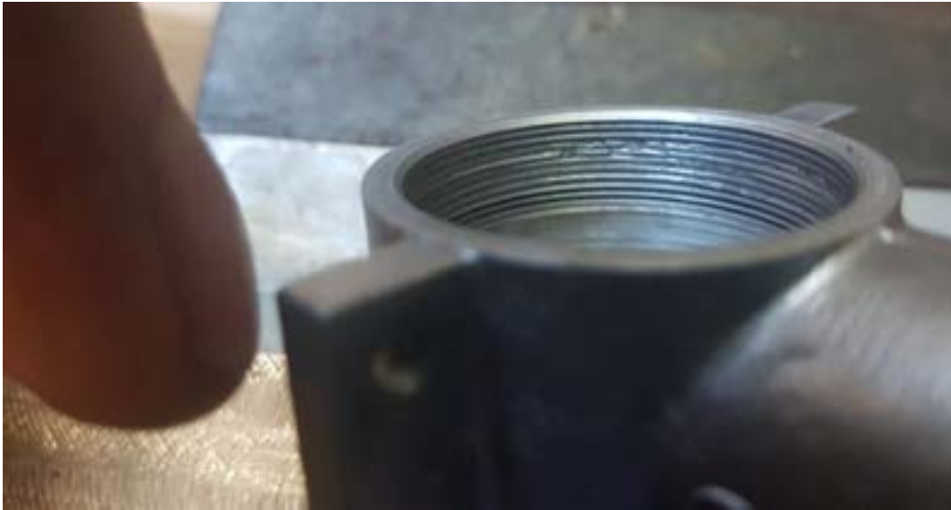
Above: Showing the crankcase galling.
