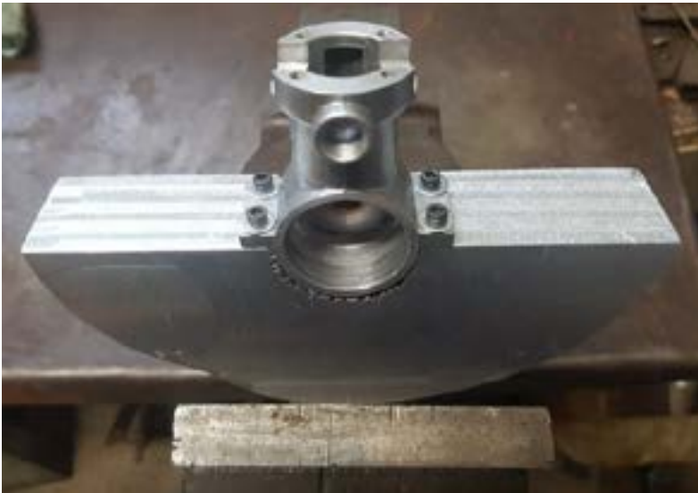
Left: Showing the engine holding fixture.
