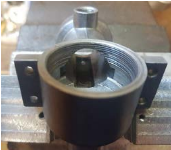
Below: Showing maximum 4 threads at the upper end of the crankcase.
