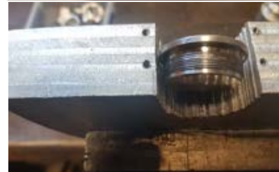
Above: Showing the back plate galling.
